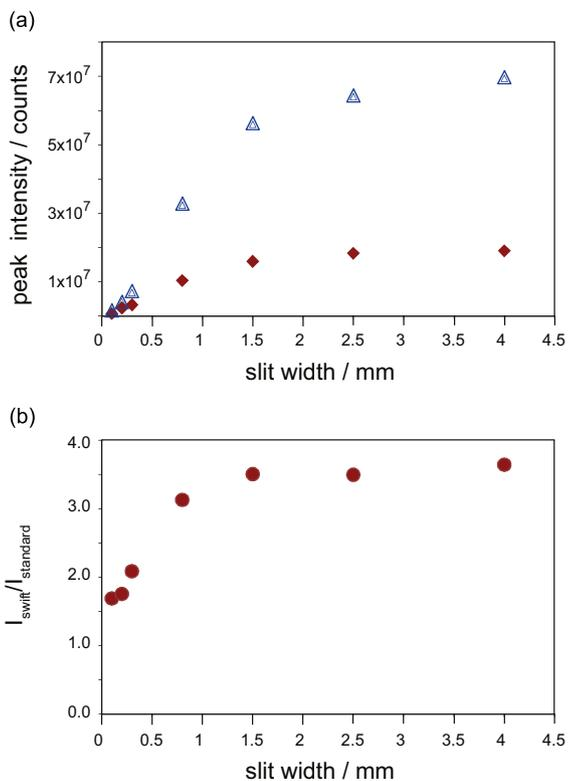
**Fig. 4.** Peak intensity (a) and peak intensity enhancement (b) as a function of slit width for the Ag  $3d_{5/2}$  peak in vacuum measurements using a pass energy of 200 eV. Data from the standard lens table and the swift-acceleration table are represented by filled diamonds and open triangles, respectively. The intensity enhancement of the swift acceleration mode compared to the standard table ( $I_{\text{swift}}/I_{\text{standard}}$ ) in figure b are illustrated by filled circles.
