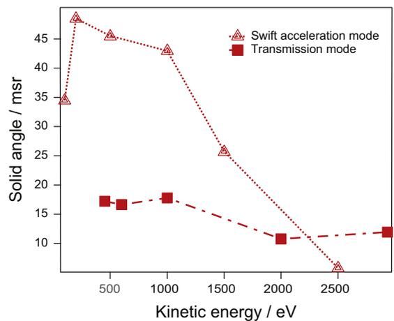
**Fig. 3.** Simulated mean solid angle collection efficiency as a function of photoelectron kinetic energy for a 0.8 mm front cone, 200 eV pass energy and a 1.5 mm slit. Data from the standard and the swift-acceleration lens tables are represented by filled squares and open triangles, respectively.
