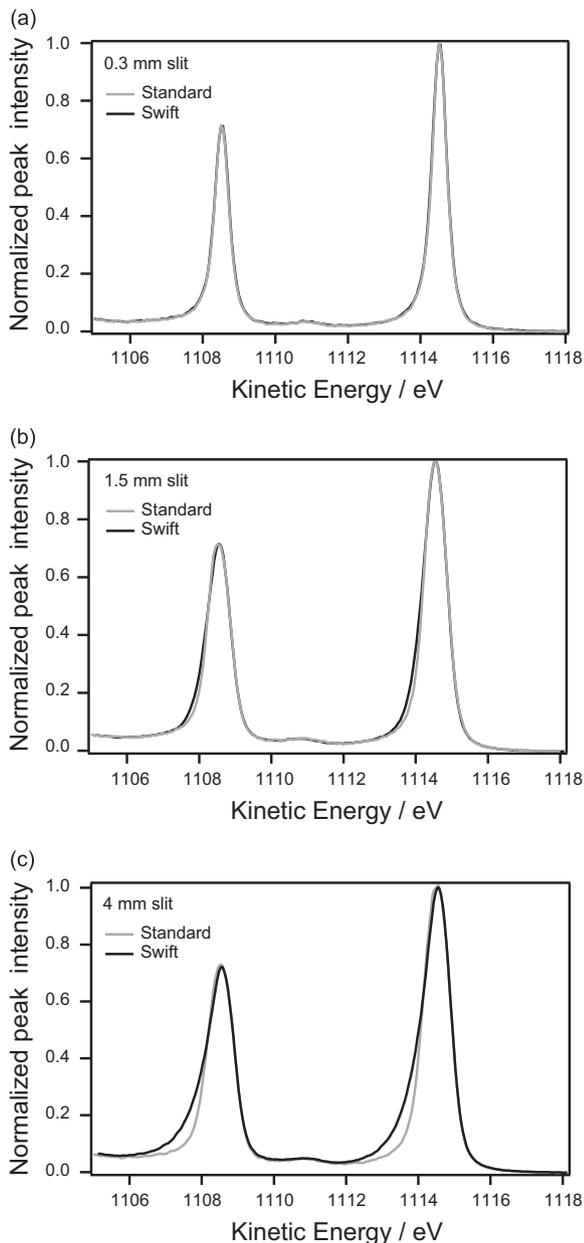
**Fig. 1.** Ag 3d peak profiles obtained with the standard and swift-acceleration lens tables in vacuum. The spectra were recorded at a pass energy of 200 eV using 0.3 (a), 1.5 (b), and 4.0 mm slits (c).
