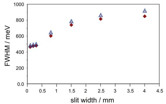
**Fig. 2.** Measured Ag  $3d_{5/2}$  resolution as a function of slit width. The measurements were done in vacuum using a pass energy of 200 eV. Data from the standard lens table and the swift-acceleration table are represented by red filled diamonds and blue open triangles, respectively. (For interpretation of the references to color in this figure legend, the reader is referred to the web version of this article.)
