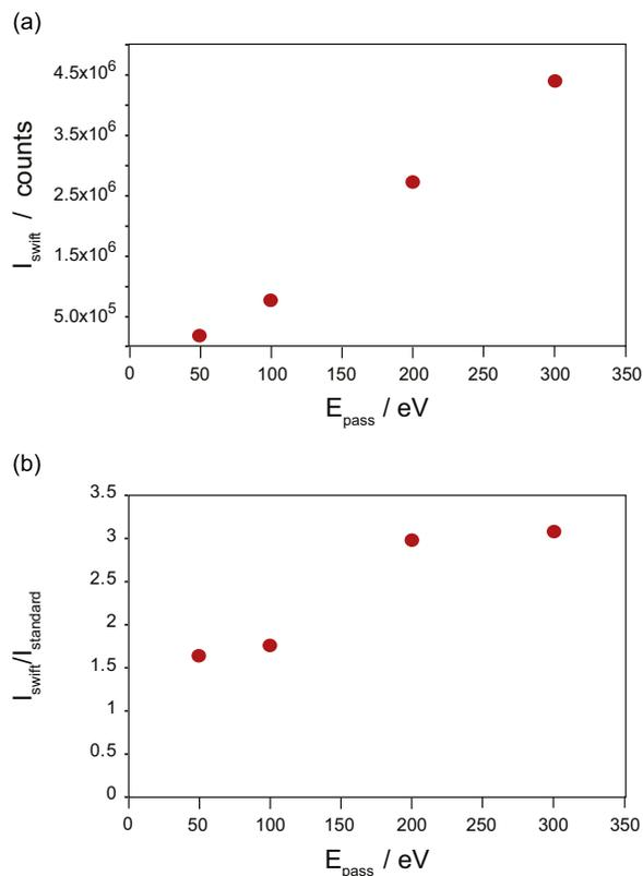
**Fig. 5.** Swift-acceleration peak intensity (a) and peak intensity enhancement compared to standard mode of operation (b), as a function of pass energy for the Ag  $3d_{5/2}$  peak in vacuum measurements using a slit width of 1.5 mm.
