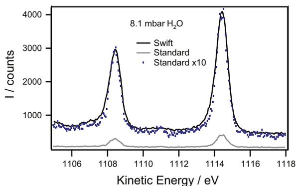
**Fig. 7.** Ag 3d peak profiles with 8.1 mbar water vapor obtained with the standard (gray line) and swift-acceleration (black line) lens tables at a pass energy of 200 eV and a slit width of 1.5 mm. In order to illustrate the enhancement of the swift acceleration mode a  $\times 10$  enhancement of the standard mode spectrum is included in the graph (blue dots). (For interpretation of the references to color in this figure legend, the reader is referred to the web version of this article.)
