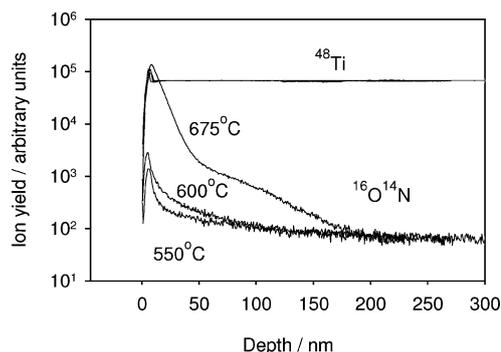
**Fig. 5** Dynamic SIMS depth profiles of  $TiO_2$  single crystals annealed in  $NH_3$  for 80 min at  $550^\circ C$ ,  $600^\circ C$  and  $675^\circ C$ . The  $^{16}O^{14}N$  ion intensity varies with depth. The  $^{48}Ti$  ion intensity is invariant after 3 nm of etching.
