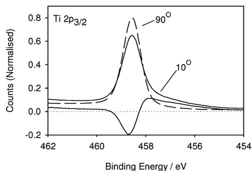
**Fig. 4** X-Ray photoemission spectra of the Ti  $2p_{3/2}$  core line recorded at take off angles of  $10^\circ$  (solid line) and  $90^\circ$  (dashed line). The peaks are normalised to the sum of the O 1s and N 1s (395.6 eV) peaks, and the difference is shown by the lower solid line.
