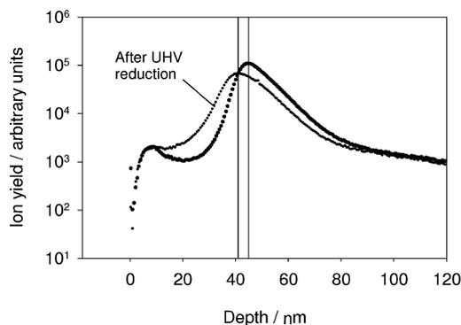
**Fig. 8** SIMS  $^{16}O^{14}N$  depth profile showing N diffusion into  $TiO_2$  (110) after 120 min of air annealing and after subsequent reduction by annealing in ultra high vacuum at 750 °C for 1 h. Vertical lines show the depths of the concentration maxima. The reduction causes migration of  $N_i$  from the bulk towards the surface.
