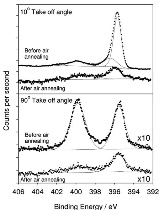
**Fig. 3** X-Ray photoemission spectra of the N 1s core line taken before and after the air annealing step at take off angles of 10° (top panel) and 90° (bottom panel). For comparison, spectra are normalised to the Ti 2p<sub>3/2</sub> core line (not shown). Data are shown as points and curve fittings, discussed in the text, are shown as solid lines.
