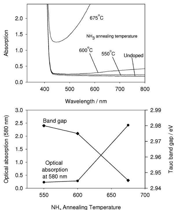
**Fig. 1** Top panel: UV/vis spectra of  $\text{TiO}_2$  (110) single crystals undoped and annealed in  $\text{NH}_3$  at 550–675 °C for 80 min. Bottom panel: variation in optical absorption intensity at  $\lambda = 580$  nm (circles) and Tauc band gap (diamonds) with annealing temperature.
